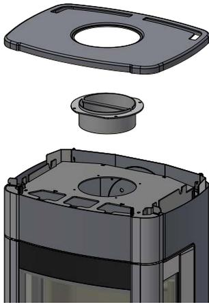
**5** Remove the cover. This is to be used later as a seal and cover at the top of the smoke outlet.
