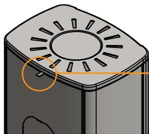
The vent for adjustment of the convection air is placed at the back of the high top
