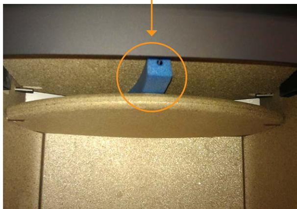
Put back the upper plate on the pins, as the protection pushes the plate upwards
