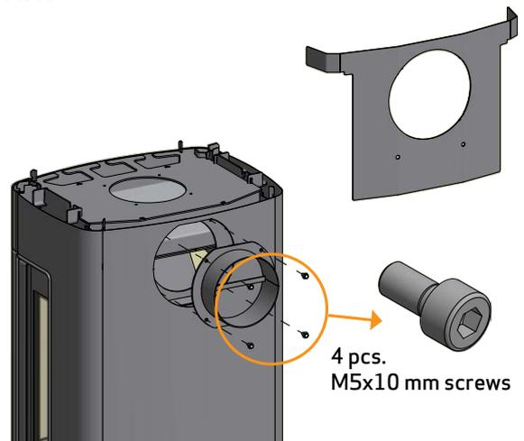
**3** Cut off the cover plate from the rear plate with cutting pliers at the fastening points
