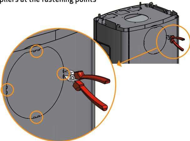
**4** Lift the heat shield off the stove and cut the cover plate free using cutting pliers at the fastening points. Remove the heat shield
