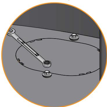
Remove the protection between the baffle plates, before taking the stove into use!
