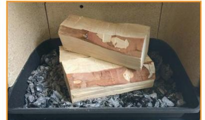
At the EN 13240-test the stove was fired as shown on the picture:
