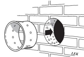
Then cement in a wall connector with fire proof mortar (not supplied). Let the mortar dry before the stove is connected to the chimney.
