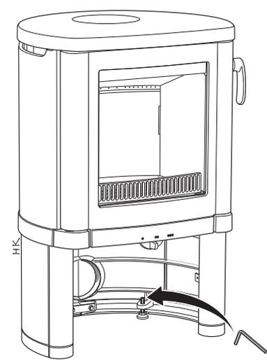
Adjust the adjustable feet until the stove is horizontal and then reinstall the cover plate.
