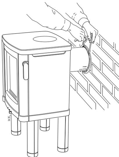
Install the connection pipe on the connection. Make sure that the gasket does not work loose from its position. Caulk between the connection pipe and the connector in the wall using caulking rope. If further sealing material is required, heat-resistant sealant may be used.
