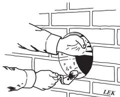
Cut a hole approximately 180 mm in diameter.
