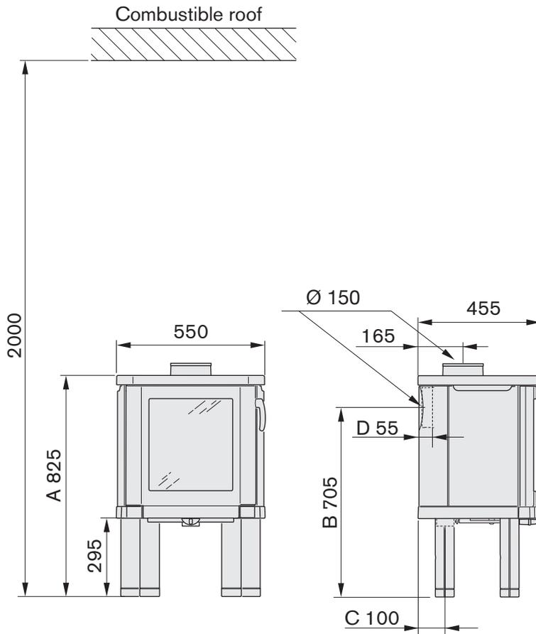
Position the stove on a hearth plate and check that the installation distances given in the diagrams are met. The minimum distance between the stove opening and combustible parts of the building or décor must be at least 1 m.
