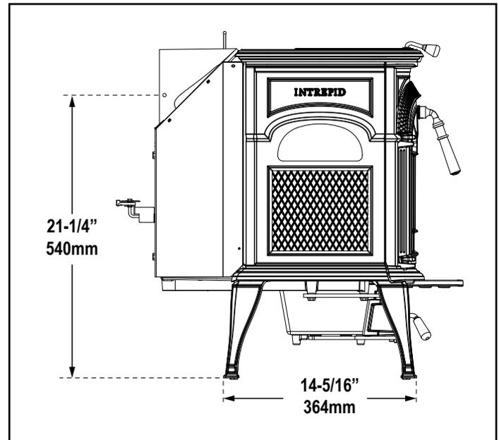
Figure 3.4 - Side View with horizontal flue
