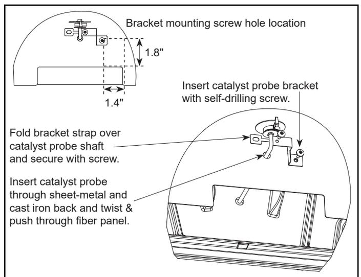
Figure 5.9 - Install the Catalyst Temperature Probe
