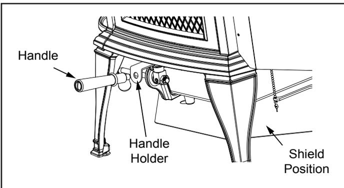
Figure 5.5 - Handle holder and heat shield positions.
