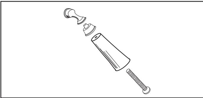
Figure 5.5 - Assemble the front door handle.
