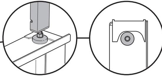
Place a spirit level on the moulding below the door, and adjust the front feet to the specified measurement from the floor to the moulding's lower edge and until the spirit level is straight.
