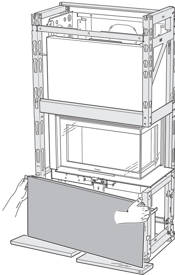
When the front panel is correctly positioned in the depth direction, it must be lowered again for the installation of the side panels. Beware of the corners!
