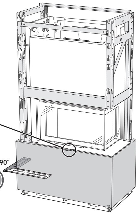
Ensure that there is a 4 mm gap between the stone and insert so that the damper can move freely.
