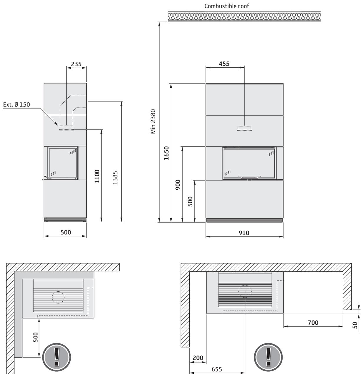
For corner installation, the rear and side walls must always be non-combustible, alternatively both must be protected by an external firewall. Material requirements for firewall according to the section "Walls behind" on page 228.
