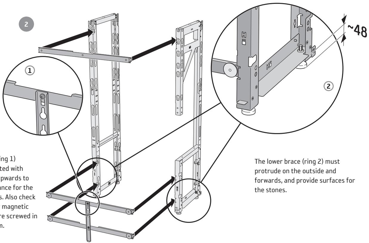
This brace (ring 1) must be twisted with the cut-out upwards to create clearance for the damper wires. Also check that the four magnetic mountings are screwed in at the bottom.
