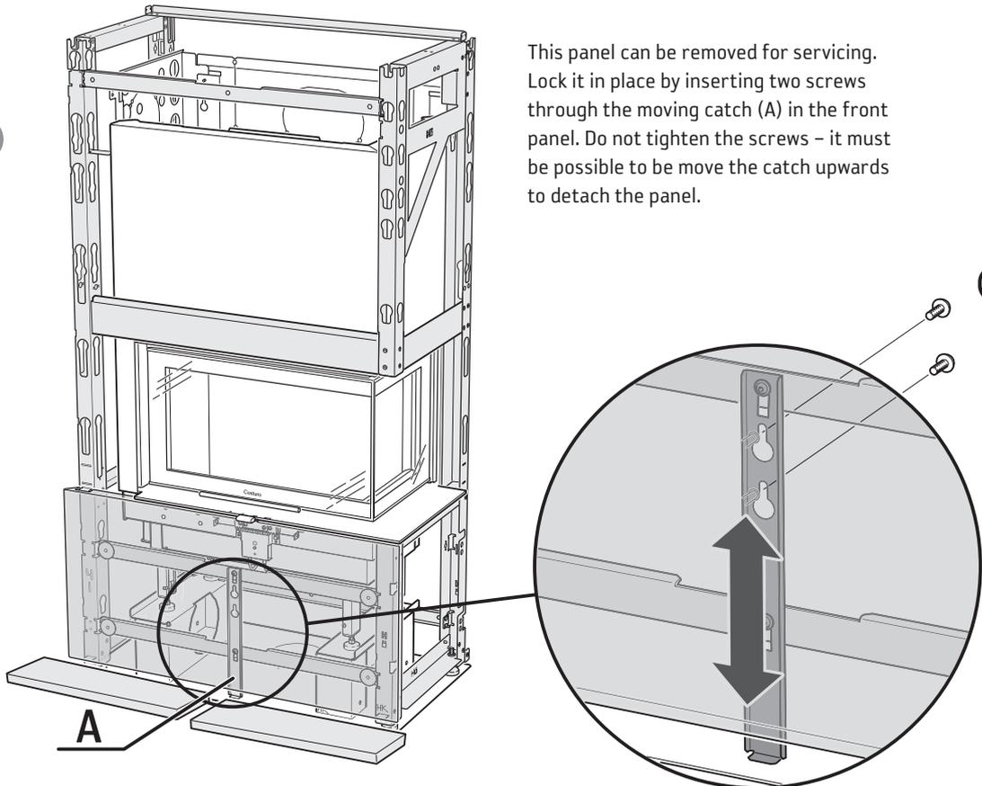
This panel can be removed for servicing. Lock it in place by inserting two screws through the moving catch (A) in the front panel. Do not tighten the screws - it must be possible to be move the catch upwards to detach the panel.
