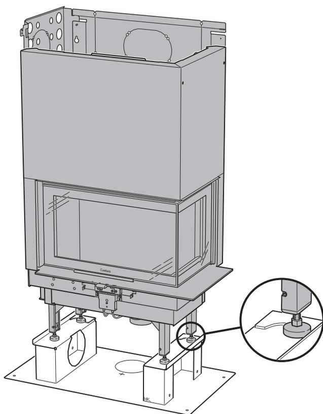
Place a spirit level on the moulding below the door, and adjust the front feet to the specified measurement from the floor to the moulding's lower edge and until the spirit level is straight.
