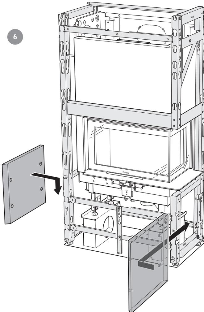
Check that the top of the stones are level using a spirit level. Use supplied shims if necessary. Carry out on the remaining stone sections.
