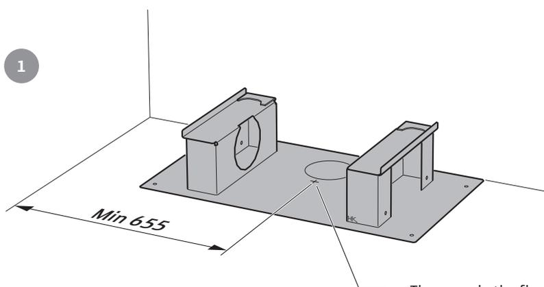
The cross in the floor panel indicates the location of the flue gas output.
