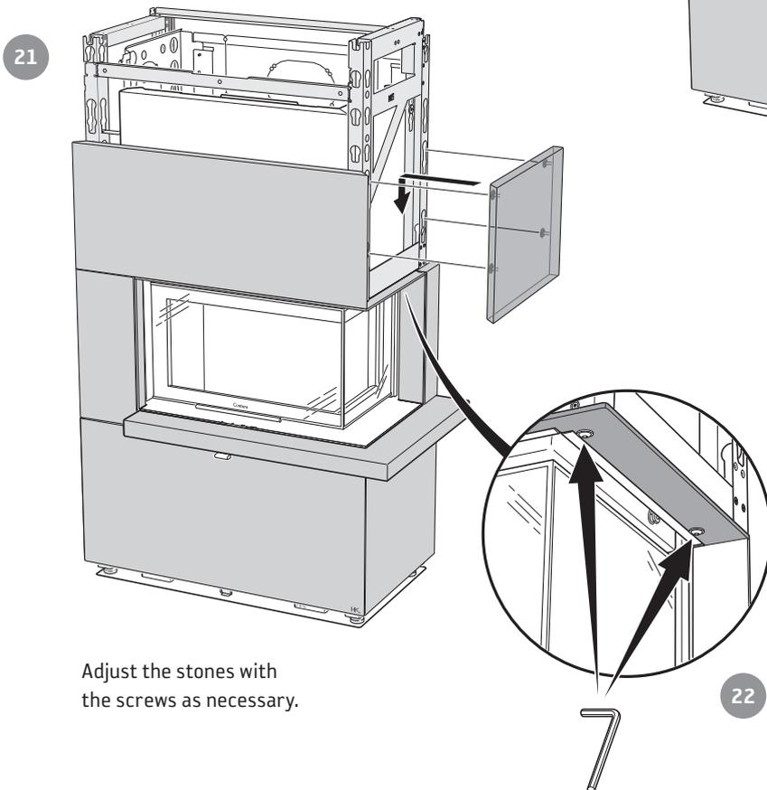
Adjust the stones with the screws as necessary.
