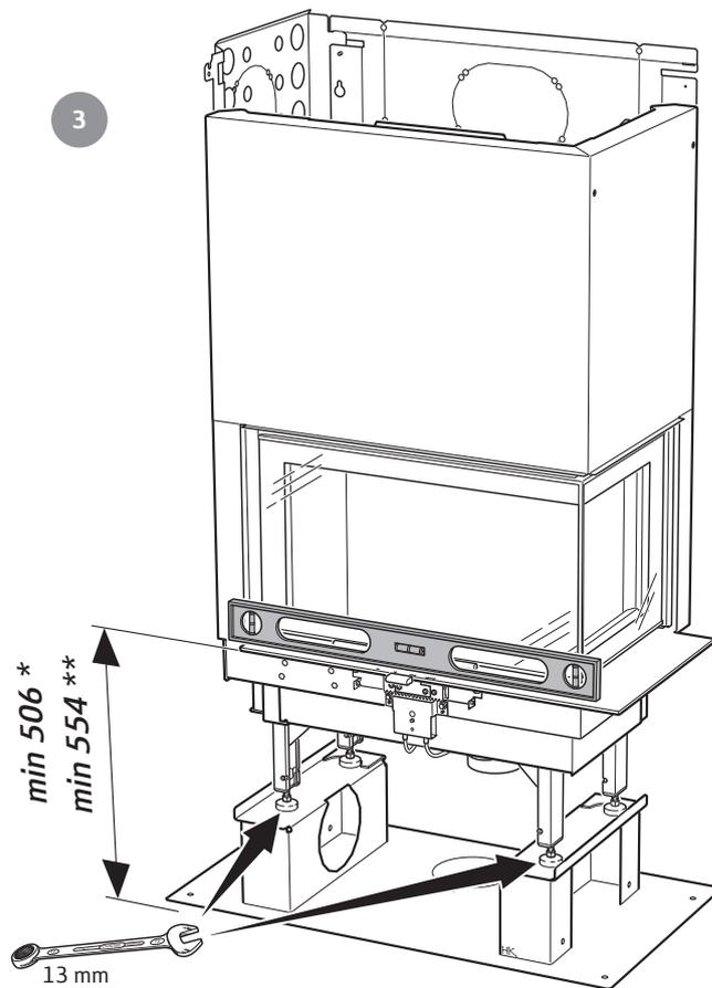
Position the spirit level as illustrated and adjust the rear feet until the stove is level.
