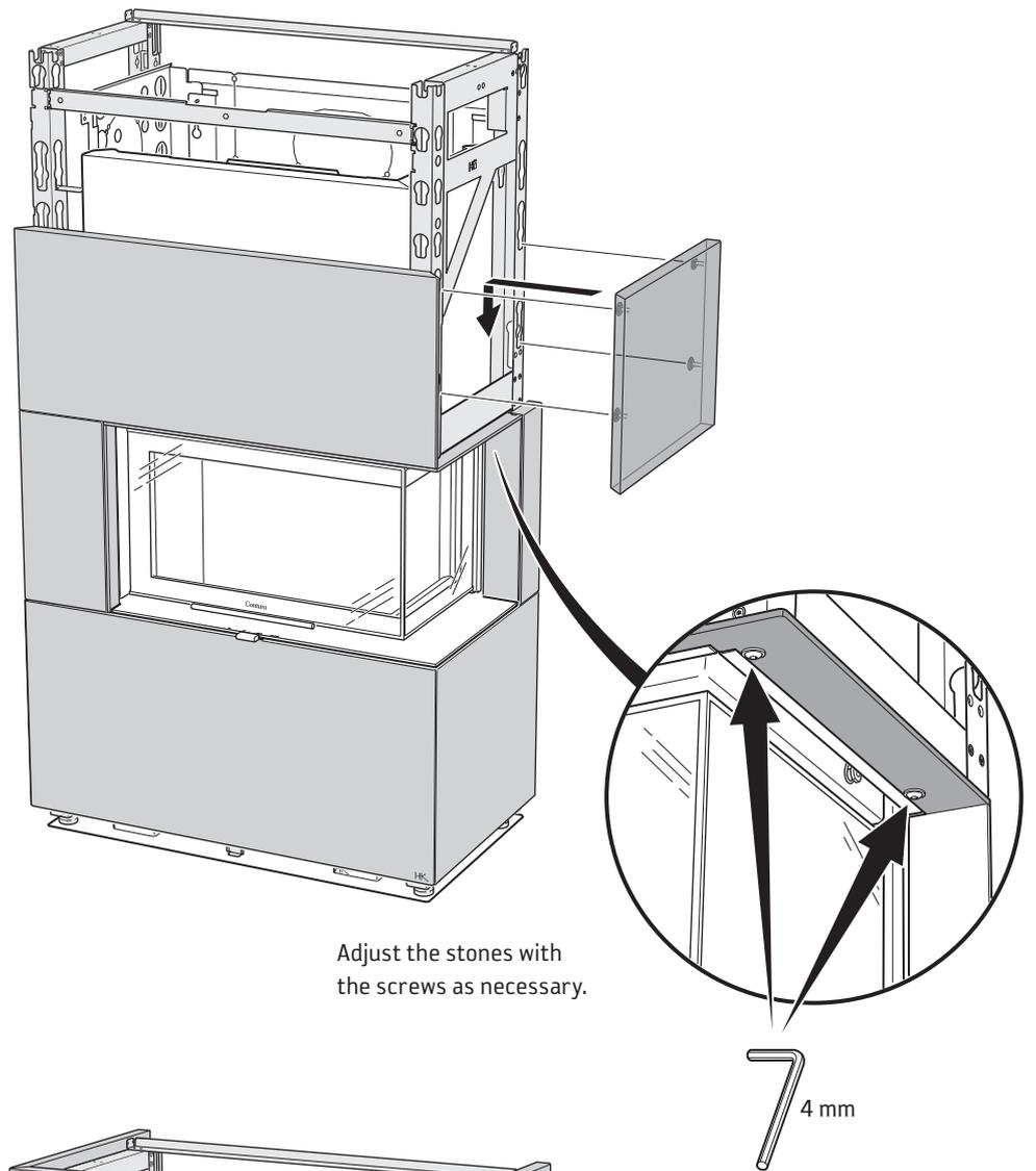
Adjust the stones with the screws as necessary.
