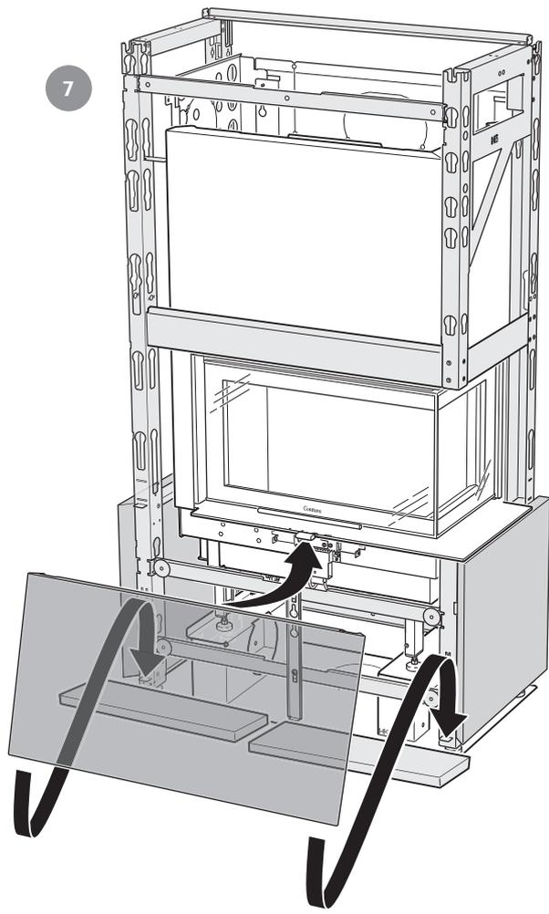
Check that the top of the stones are level using a spirit level. Use supplied shims if necessary. Carry out on the remaining stone sections.
