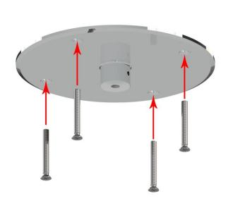
**STEP 2** - Secure the Fixed Ceiling Base to the load bearing surface using steel screws or bolts, depending on the structure it is being secured to (fasteners are not provided). The holes in the Fixed Ceiling Base are Ø7mm.
