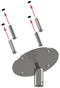
**STEP1** - Mark and drill 4 holes into the load bearing surface and insert the corresponding metal anchor dowels into the holes (fasteners are not provided). The holes in the Angled Ceiling Base are Ø7mm.
