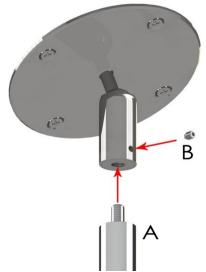
**STEP 4** - Screw in Extension Poles or Stainless Steel Hanging System (A) into the corresponding threaded hole in the Angled Ceiling Base and secure it with the Security Screw (B). The height adjustment of the Stainless Steel Hanging System is the same as indicated for the Fixed Ceiling Base.
