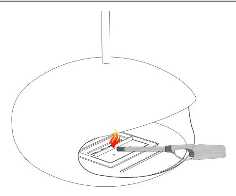
Using a long arm fire lighter and standing at a safe distance from the Combustion Chamber carefully introduce a flame as indicated above to ignite the Combustion Chamber. Always make sure there is a Class ABE fire extinguisher close at hand when igniting the Combustion Chamber.
