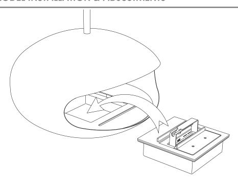
With the Mount Plate in the correct position and secured in place with the hex nut, the Combustion Chamber can now be placed inside and taken off the Mount Plate opening using the Lifting Handles supplied as shown on the previous pages.
