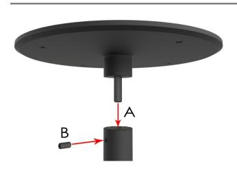
**STEP 3** - Screw in Extension Poles (A) into the corresponding threaded hole in the Black Fixed Ceiling Base and secure it with the Security Screw (B).
