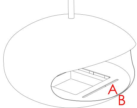
NOTE: adjustment instructions on the following page showing relative positions of (A) and (B) shown above are critical to the airflow inside the *Main Body* and therefore critical to the proper functioning of the *Combustion Chamber*.
