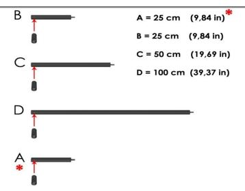
STEP 4 - The finished height of the Black Hanging System is made up of a combination of the Extension Poles (B, C & D). The Connection Pole (A) is NOT OPTIONAL\* and must be connected to the Main Body with the washer, hex nut and wing nut supplied.
