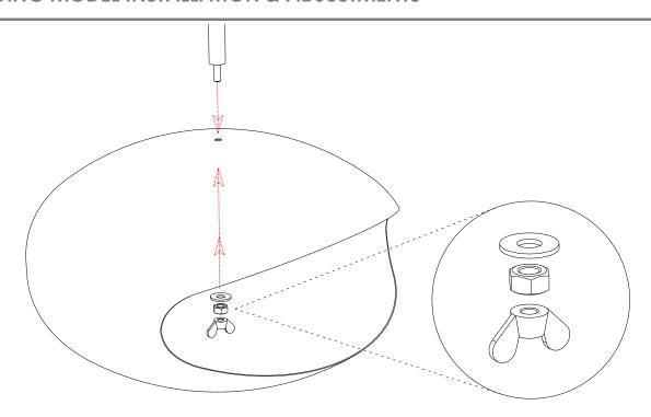
Position the Main Body onto the threaded end of the Connection Pole and secure from inside with first the washer, then the hex type nut and finally the wing type nut.
