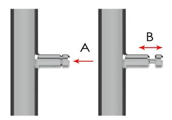
**STEP 4** - Adjust the height of the extension bar system by pulling the security pin on the side and raising or lowering the bar. fig (A) shows the security pin on the locked position.
