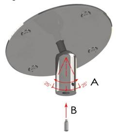
**STEP 3** - The Stainless Steel Angled Ceiling Base allows for a maximum angle of 25 degrees, this is the maximum angle the load bearing surface. Once the fixing collar (A) is vertical, secure in place with Safety Screw (B).
