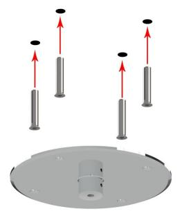
**STEP1** - Mark and drill 4 holes into the load bearing surface and insert the corresponding metal anchor dowels into the holes (fasteners are not provided). The holes in the Fixed Ceiling Base are Ø7mm.
