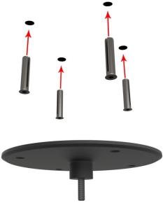
**STEP1** - Mark and drill 4 holes into the load bearing surface and insert the corresponding metal anchor dowels into the holes (anchor dowels are not provided). The holes in the Black Fixed Ceiling Base are Ø7mm.
