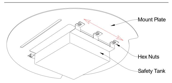
Further adjustment to the position of the Mount Plate can be achieved by loosening the 6 hex nuts below the Mount Plate and sliding the Safety Tank front to back slightly. Always make sure that the Safety Tank below the Mount plate is properly secured after this adjustment.
