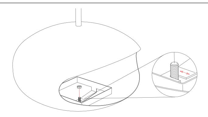
Position the Movable Tray Bracket over the threaded stud at the base of the Main Body and adjust according to the instructions on the following page before securing with hex nut.
