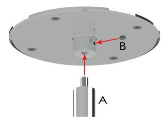
**STEP 3** - Screw in Extension Poles or Stainless Steel Hanging System (A) into the corresponding threaded hole in the Fixed Ceiling Base and secure it with the Security Screw (B).
