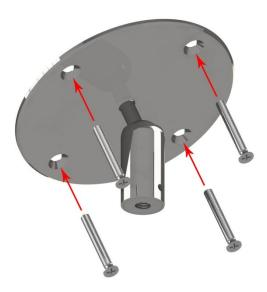
**STEP 2** - Secure the Angled Ceiling Base to the load bearing surface using steel screws or bolts, depending on the structure it is being secured to (fasteners are not provided). The holes in the Angled Ceiling Base are Ø7mm.
