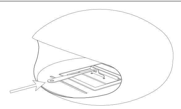
To extinguish the flame, insert the tips of the *Sliding Lid Handle* into the holes of the *Sliding Lid* of the *Combustion Chamber* and slide all the way forward until the flame is extinguished. Should the flame not extinguish with the first try please repeat until extinguished. **It should be a swift action coupled with downward pressure**.
