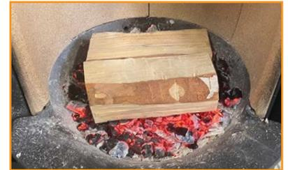
At the EN 13240-test the stove was fired as shown on the picture:
