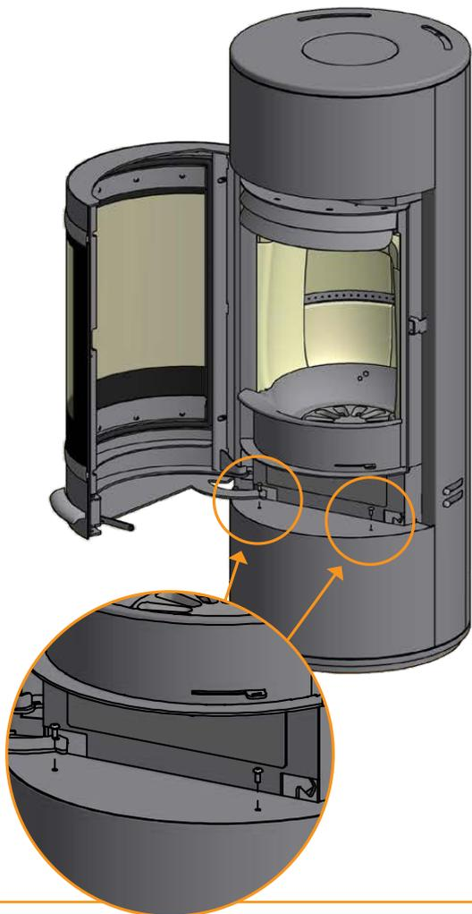
Adjust the adjustment screws
