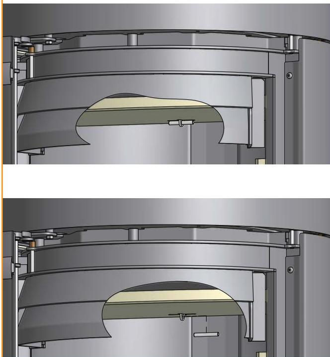
The baffle plate holder may fall out when the baffle plate is taken out of the stove. See the illustrations below for how to fit it
