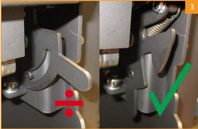
Over time, the door may “hang” a little. You can correct this by pressing the locking device upwards by means of an adjustable spanner.
