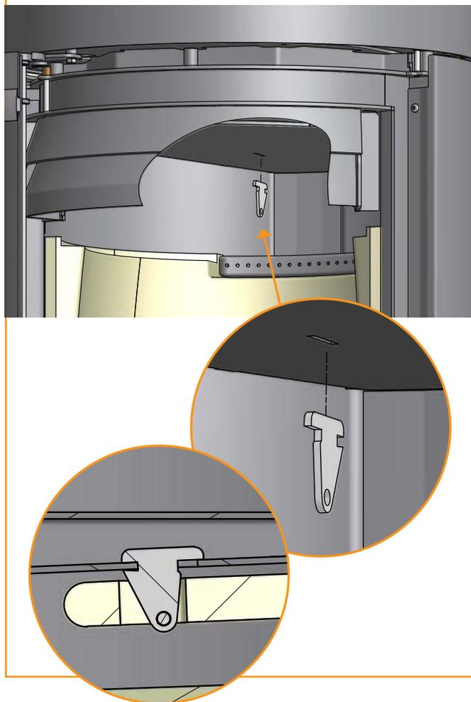
Pass the baffle plate edge-first and downwards out through the combustion chamber
