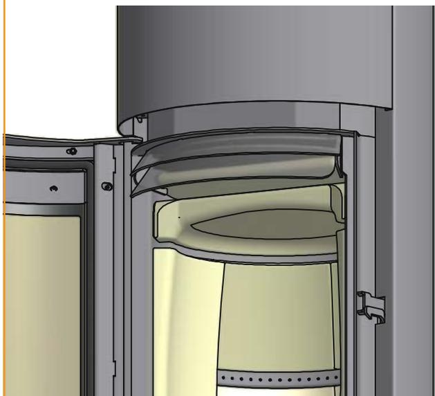
Turn the baffle plate 90°, and lower it out through the combustion chamber
