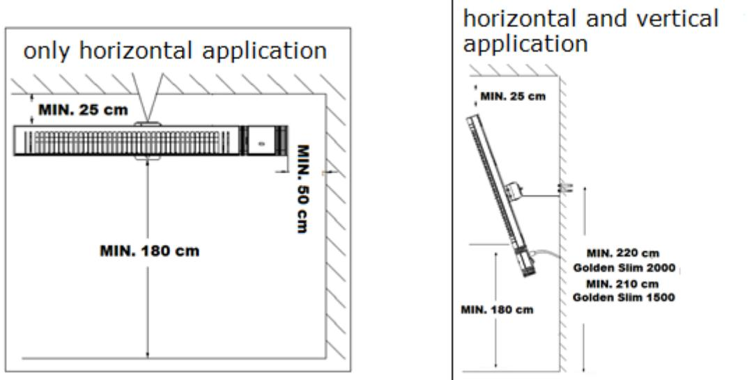
The Golden Slim infrared heater is equipped with a rotatable wall bracket so that it can be used horizontally or vertically. This deserves special attention when installing the appliance, because you must take into account the minimal distances from the wall, ceiling and ground in all the optional positions:
